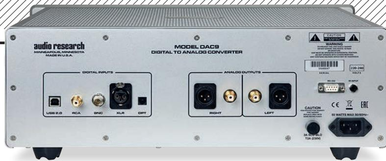
ABOVE: A single set of RCA and (balanced) XLR analogue outs lie alongside optical, BNC and coax (S/PDIF) and XLR (AES/EBU) digital inputs. RS232 services automation
